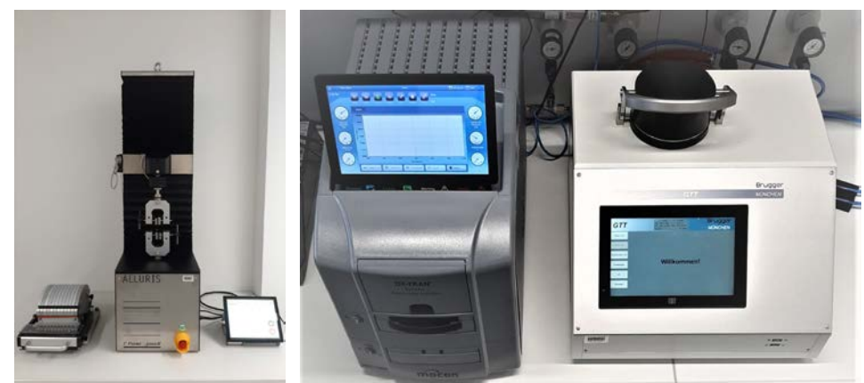
Figure 2: Tensile testing, Gas and Oxygen-Permeation-Testing ( Itr )
