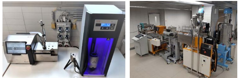
Figure 1: Lab-Compounder & -Injection moulding, Pilot-scale compounder and flat film extrusion line ( Itr )
